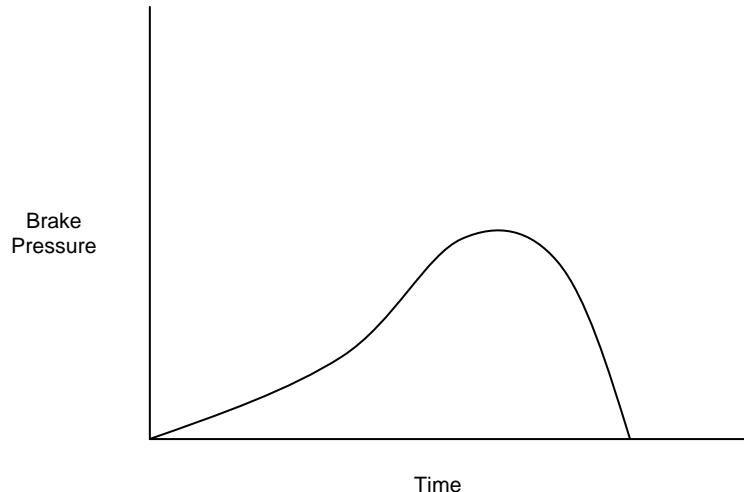
At the same time, we want to keep our braking distances as short as possible, so we can go faster around the racetrack. How do we accomplish both of these? By inverting the whole braking technique – by braking hard in the early part of the braking maneuver, and reducing pedal pressure as we come off the brake.
